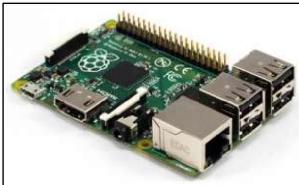
**Gambar 2. 7. Raspberry Pi 3 Model B+**
