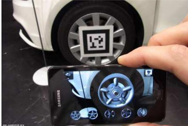
**Gambar 2.19** *Marker Based Augmented Reality*
